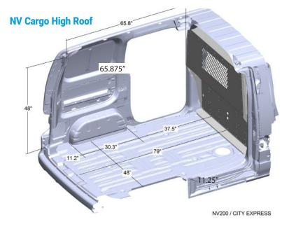
\* Measures 79" at the floor and up to 13" off the floor. Measures 72" at 23" and higher off the floor.
