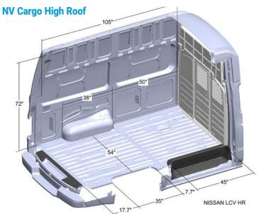
\* Subtract 3" from dimension when a Max Comfort partition wing kit is installed.
